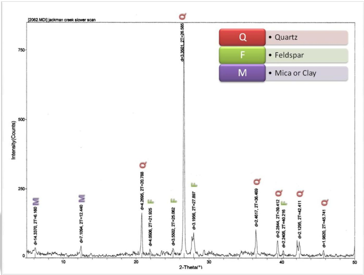
Figure 4: X-Ray Diffraction showing the concentrations of Quartz, Feldspar and Mica/Clay.
